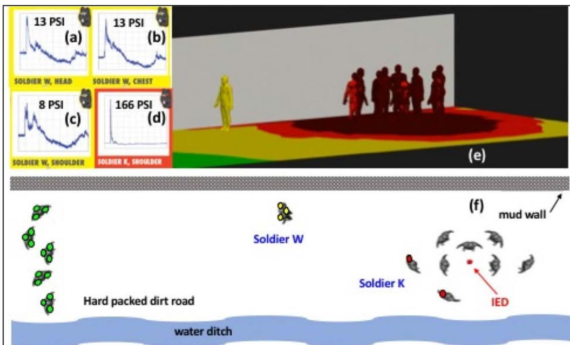
Blast gauge data, coupled with contextual data of the event from soldier interviews, was used to build a computer simulation to recreate the blast pressure wave from an IED attack. Figures (a-d) show actual measurements of blast gauges worn on soldiers in the attack; (e) shows the computer simulated blast exposures of soldiers from the event recreation; (f) shows the soldiers' location.
