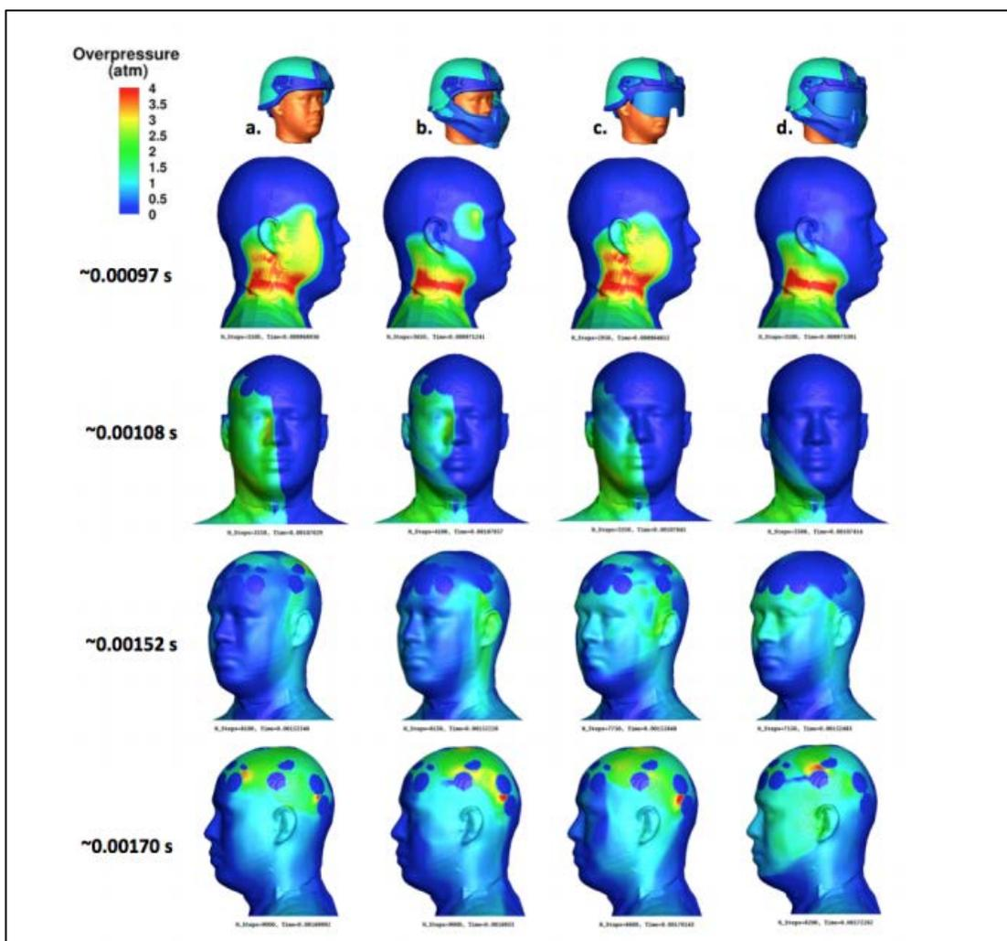
Computational modeling shows the peak pressure differences and locations over time for various helmet configurations as side-initiated blast waves travel through the head. Different helmet configurations can produce different patterns of blast pressure propagation in the head and brain.
